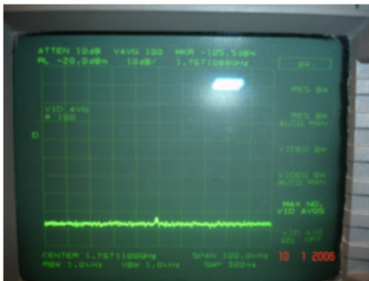
Second harmonic response of diode in normal configuration
